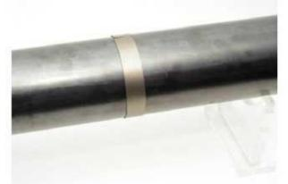
Attach for electromagnetic isolation "Ferrite Tape" 2 x one layer around the shaft.
