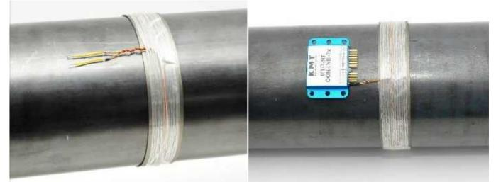
Extend the CUL wire flexible 0.14-0.25 mm (to decouple Twist also the flexible wire and solder it on the MTP-NT the inflexible 1 mm wire, at 0.63 not necessary) IND-Tx (isolate all solder points with shrink tubing)
