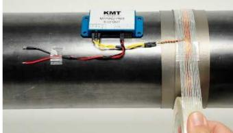
Solder the end of the wire on the AC IN of the IND-PWR module and isolate all solder points with shrink tubing.
