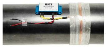
**Note:** "The inductive load of the MTP-NT IND-PWR and the capacitor in the Power Head must be in resonance to get the optimal transmission. The inductive load of the shaft depends of diameters, material and number of windings!
