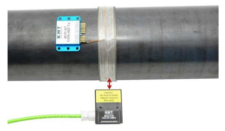
Inductive Pick-Up head mount in this position! Distance between head and Tx coil can be up to 50 mm, distance deepens of application.
