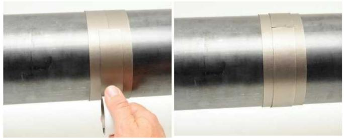
Attach for electromagnetic isolation "Ferrite Tape" 2x parallel and 1x in the middle over two layer around the shaft
