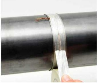
Make transmitting coil with 1x winding and twist the end of wire. Use CUL 0.63-1.00 mm wire
