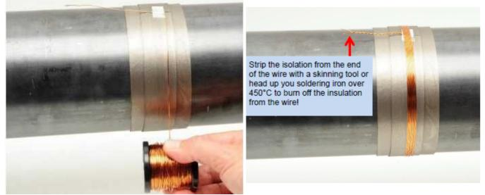
Make power coil with 3-18 windings for 1000-20 mm diameter (see diagram) and twisted the end of wire. Use 0.63...1.00 mm (1.00 mm for diameter of 100-1000 mm) CUL wire (Enameled copper wire)
