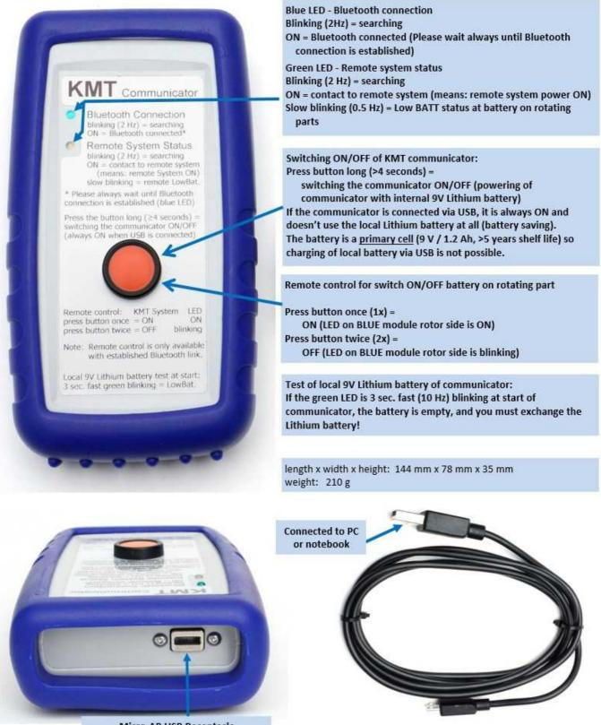
Micro-AB USB Receptacle for powering and communication to PC When connecting the USB port, a Windows COM port is created automatically. A driver doesn't have to be installed; we use the FTDI FT230X chip, which is always automatically recognized by Windows.
