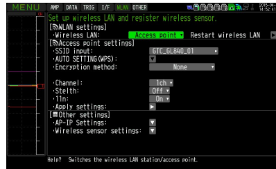
Access point settings
