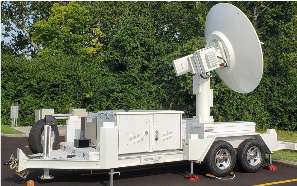
Digital Antenna - RF arrives, IP packets delivered
