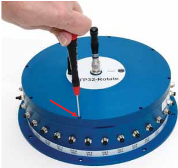
1. Open hexagon screw (2.5mm) with 2mm screw driver
