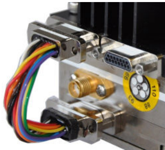
Connection to transmitter with a female MDM-15
