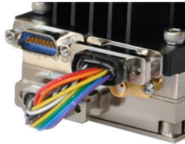
Connection to transmitter with a male MDM-15
