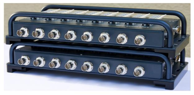
Additional BNC input connectors for differential voltage inputs allow to connect voltage signals to every amplifier input directly without disconnecting the break-out box cable from the system.
